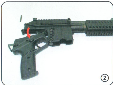
插梢取出後，即可將上下槍身分離 Upon removal of the Assembly Pin, rotate Pistol Grip down and forward for separation.
