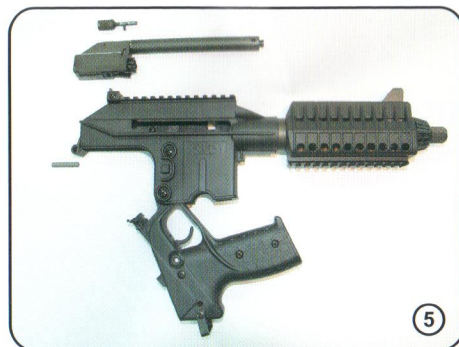
大部分分解完成 Majority of the rifle is disassembled.
