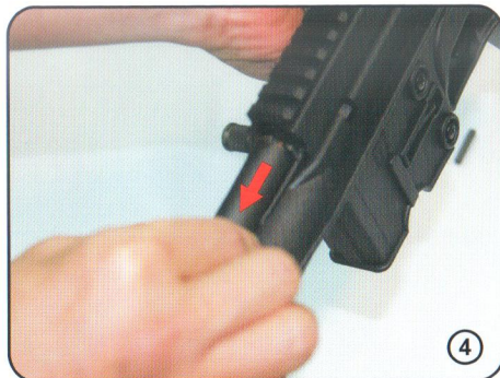
欲取出槍機，先將槍機前桿拉出90°往前推出 To remove the Bolt Carrier Group, pull the Gas Piston Rod towards to the muzzle and rotate left 90°. Then pull the Charging Handle all the way back.
