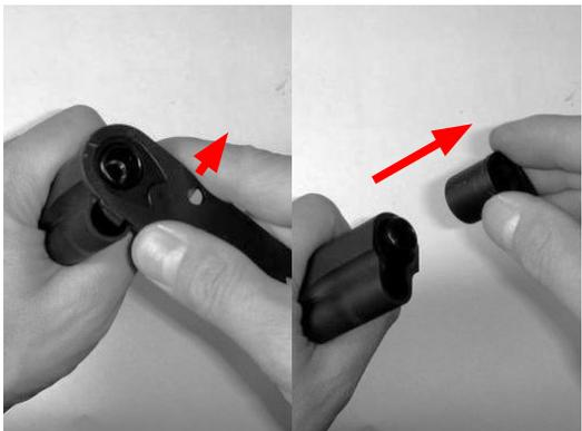
USE WRENCH TO ROTATE THE BARREL BUSH AND REMOVE IT
