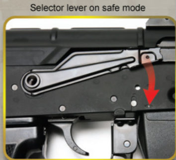
Selector lever on safe mode. Turn the Selector Lever to Auto or semi mode.
